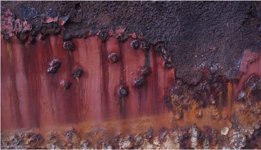
Figure 3 Water-line oxidation suggesting layers of decay. (Screenshot from Ghost ships of Suva , 2020; photo by the author.)
